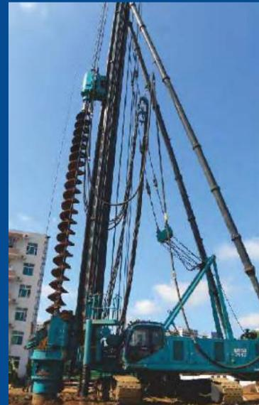
SWSD series drilling rigs with double power heads
