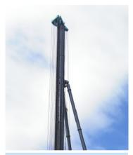
The diameters of the column and the support rod are 1,020mm and 610mm respectively, which can significantly improve the strength and reliability of the machine. The maximum mast height can reach 60m (when custom-made).
