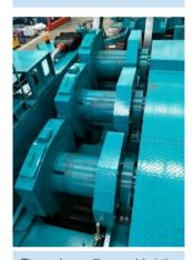
The main, auxiliary and hoisting winches have the free release function, and the whole machine is equipped with 6 winches, making it suitable for various construction methods.
