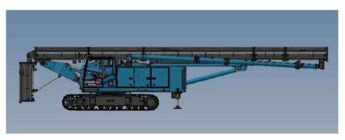
• 整机配置4个卷扬机组,功能全面。 Four winches is equipped to offer all-around functions.
